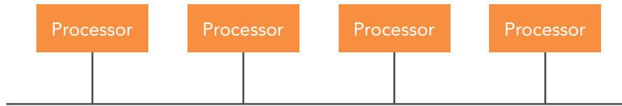
Figure 10.2: With SMP, each processor run threads from both user applications and threads belonging to the operating system
