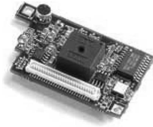
Figure 15.3 MTS310 sensor board with on-board microphone seen at the top left corner of the board.
